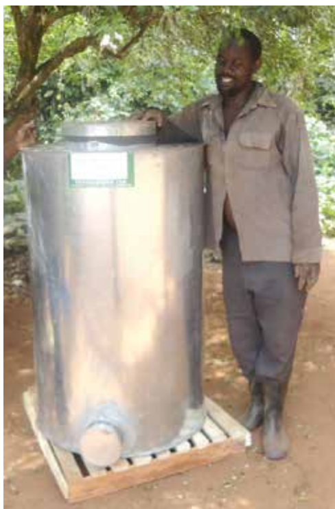
Figure 3.1: A farmer with a metallic grain seed storage silo for hermetic preservation.
